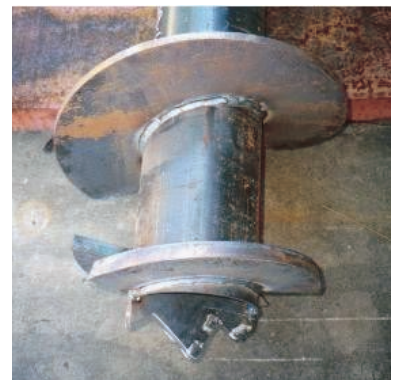
(Below) Rock bit welded to the screw pile
